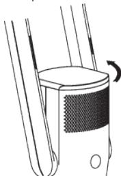
1. Turn the filter system top cover counterclockwise to unlock and remove the filter.
