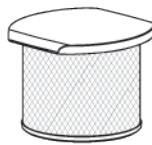
3. The new filter and top cover are attached and assembled with a buckle.
