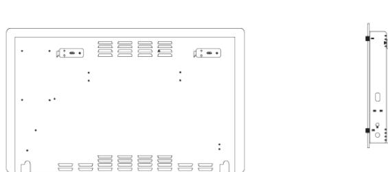
3. Hold the side of the product, look at the position of the wall hole on the rear cover, and slide to the top of the slot. This means the wall installation is complete, as shown in the picture below.
