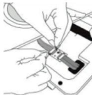
• **Step 3:** Pull out the HEPA filter screen directly by pulling up with both hands (Figure 4), to replace it, note the direction of the arrow labeled on the filter screen (Figure 5).
