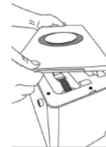
• **Step 2:** Gently move the loosened panel to the side of the purifier body, then gently pull the panel away from the FFC cable buckle of the main body with your fingers, and then hold the panel open. (see Figure 3)
